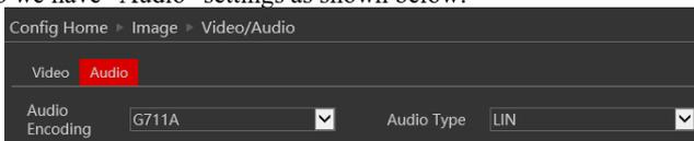
Set the encoding profile as desired and the type of audio input. If LIN (Line) is selected, it means that the audio input is already amplified and the input volume will be set to "low". If MIC (Microphone) will be
