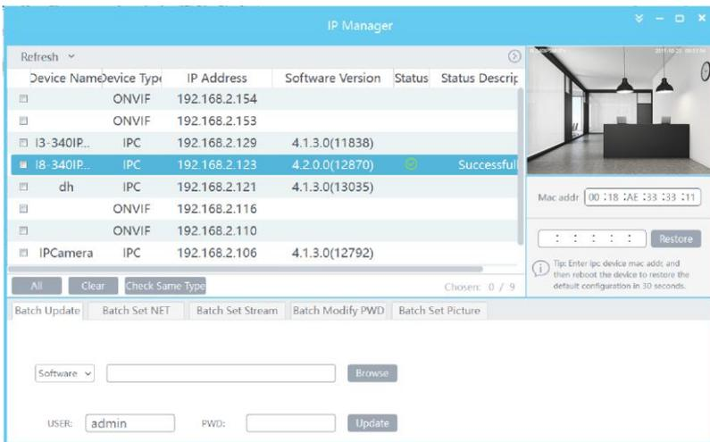
③ Modify the IP address. The default IP address of this camera is 192.168.226.201. Tick all the cameras you wish to set and then click on the “Batch Set NET” tab.
