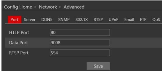
The screenshot shows the configuration page for the 'Port' section. The breadcrumb trail is 'Config Home > Network > Advanced'. The 'Port' tab is selected. The configuration fields are:
