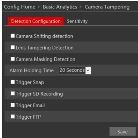
2. Enable the required detection analytics out of Camera Shifting/Lens Tampering/Masking detection.
