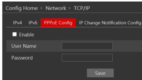
The screenshot shows the configuration page for PPPoE. The breadcrumb path is "Config Home > Network > TCP/IP". There are four tabs: "IPv4", "IPv6", "PPPoE Config" (highlighted in red), and "IP Change Notification Config". A checkbox labeled "Enable" is checked. Below the checkbox are two input fields: "User Name" and "Password". A "Save" button is located at the bottom right.
