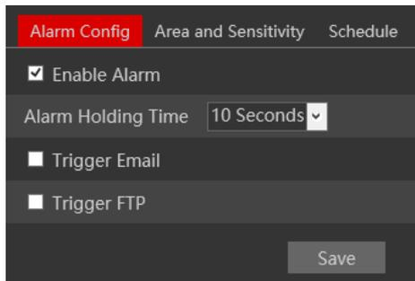
The first tab is the “Alarm Config”. Enable or disable the alarm and set the alarm holding time. The holding time means that the alarm signal will stay active and no additional alarms will be generated during that time.
