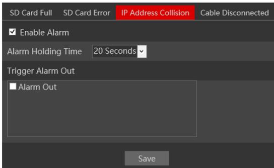
After enabling the alarm, choose the responses required from the camera in case the alarm will be active. Note that any response related to the network such as email or FTP is not available since in most cases the network will become unavailable for the camera. After the setting is complete, click “Save”.
