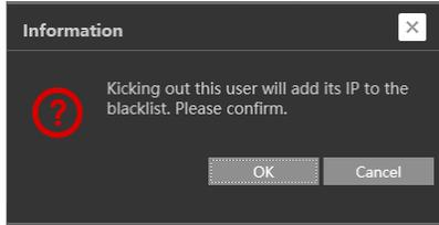
**Important Note:** once the user is kicked out, the IP address used for connection will be blacklisted. Therefore, the device used for connection will not be able to connect to the camera until the IP address will be manually removed from the blacklist.
