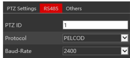
**\*Please Note:** All parameters must match exactly the setting of the analog controlling device. Otherwise, the camera will not respond.
