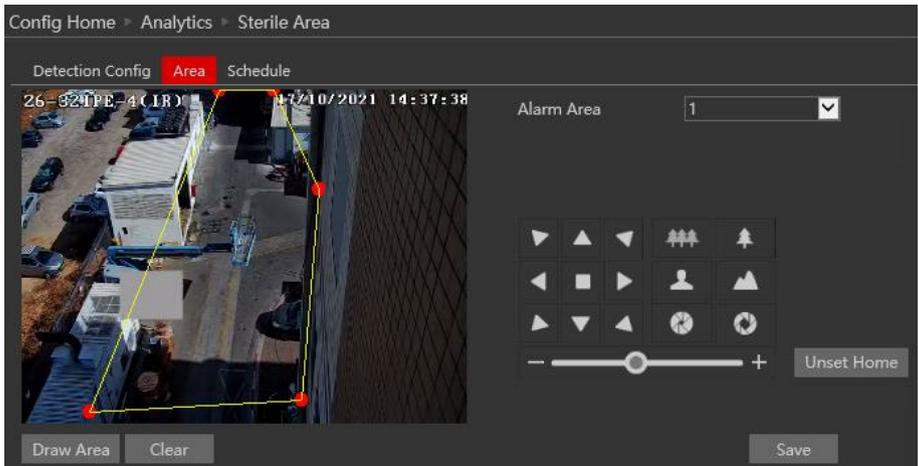
7. Move the PTZ to the desired location using the PTZ controls
