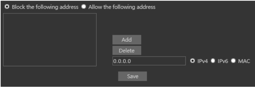
Enable the filtering you wish to activate. For the demonstration, we will enable both IP and MAC filtering, so the instructions below are true for both.
