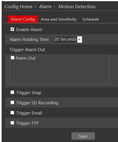
The first tab is the “Alarm Config”. Enable or disable the alarm and set the alarm holding time. The holding time means that the alarm signal will stay active and no additional alarms will be generated during that time.
