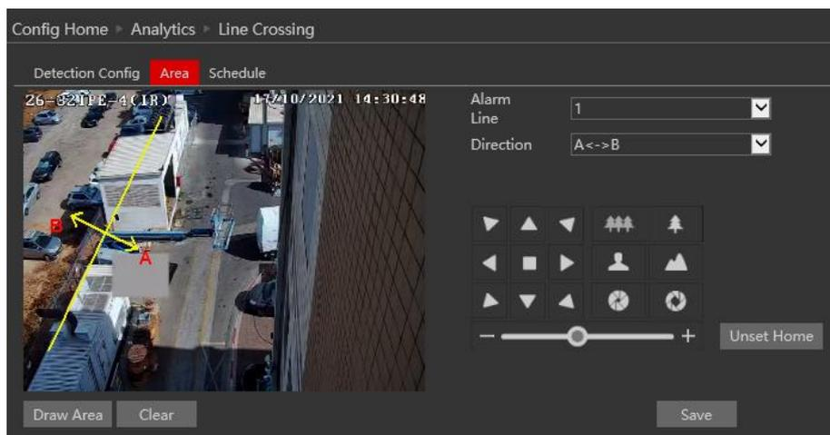
7. Move the PTZ to the desired location using the PTZ controls
