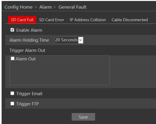
After enabling the alarm, choose the responses required from the camera in case the alarm will be active. After the setting is complete, click “Save”.
