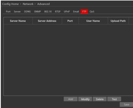
To add a new FTP server click on “Add” and input the FTP server’s server name, address, port number, username, password, and upload path, click OK to confirm the setting.
