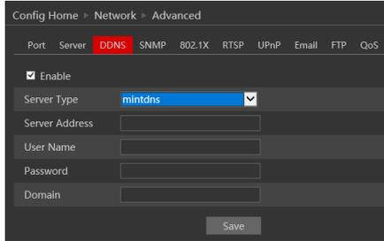
The screenshot shows a web interface for configuring DDNS. The breadcrumb path is "Config Home > Network > Advanced". The "DDNS" tab is selected. The interface includes a "Server Type" dropdown menu set to "mintdns", and input fields for "Server Address", "User Name", "Password", and "Domain". A "Save" button is located at the bottom right.
