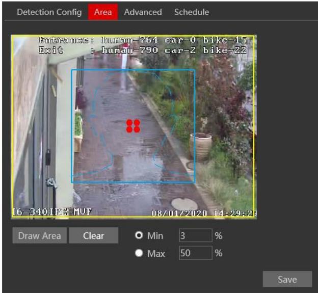
6. Set the Detection area as well as the minimum and maximum face size for detection. Click on “Save” to confirm.
