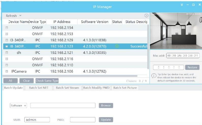
③ Modify the IP address. The default IP address of this camera is 192.168.226.201. Tick all the cameras you wish to set and then click on the “Batch Set NET” tab.
