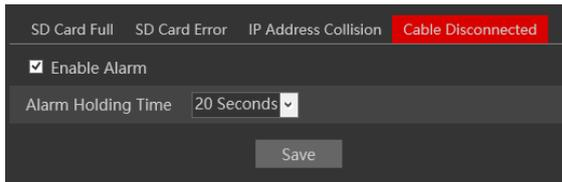
The screenshot shows a configuration interface for the Cable Disconnected alarm. At the top, there are four tabs: "SD Card Full", "SD Card Error", "IP Address Collision", and "Cable Disconnected" (which is highlighted in red). Below the tabs, there is a section for "Cable Disconnected" with the following options:
