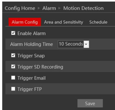
The first tab is the “Alarm Config”. Enable or disable the alarm and set the alarm holding time. The holding time means that the alarm signal will stay active and no additional alarms will be generated during that time.
