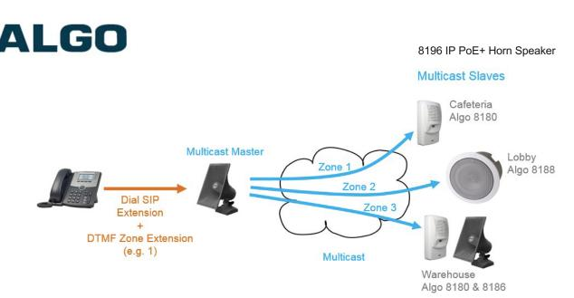
In 'DTMF Selectable Mode', to page, dial the SIP extension of the master device: ####, then dial the desired DTMF page zone (e.g. 1, 2, etc.) on the keypad when prompted.
