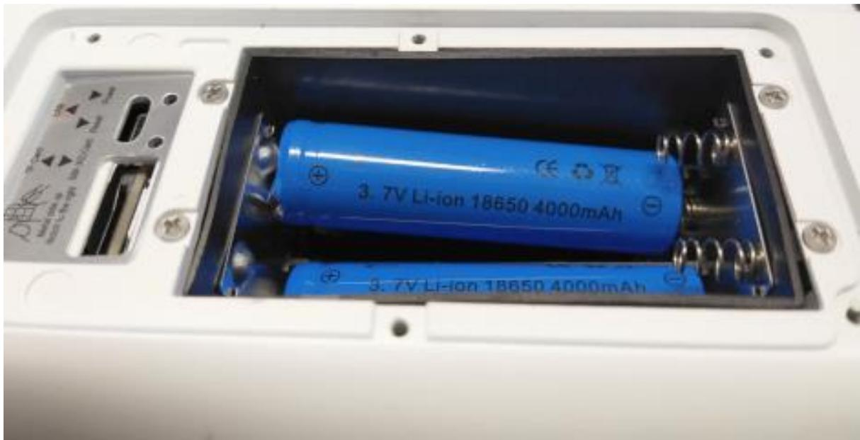
Optional – A USB A to Micro USB cable may be installed to the device to charge the batteries and apply power where no batteries are installed.
