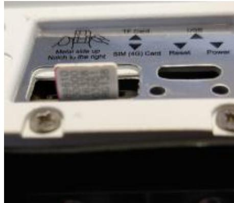
When the SIM card is fully inserted, a click will be heard and the SIM will not spring back.
